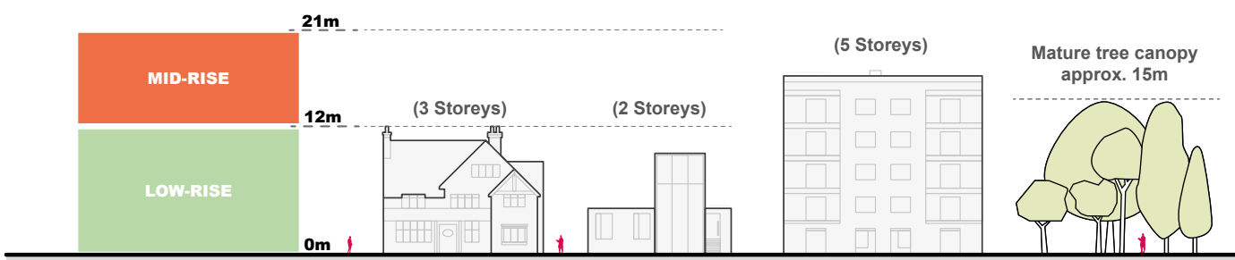
Figure 5. A diagram illustrating what low rise buildings, up to 12m, and mid-rise buildings from 12m to 21m, looks like in Kingston.
