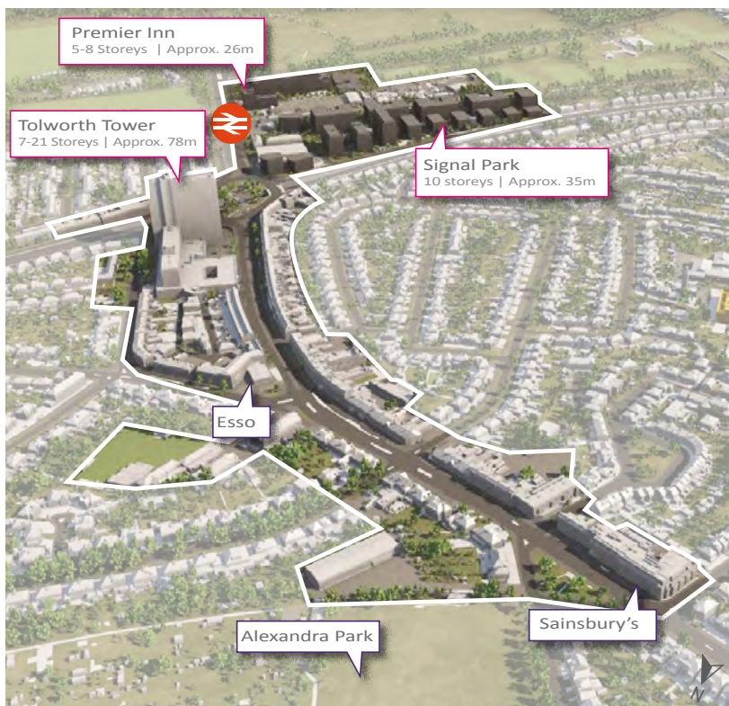
Figure 19. 3D map showing building heights in Tolworth of both existing buildings and those approved but not built.
