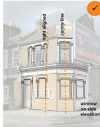
Preferred arrangement. Lower floor windows are aligned with the upper floor and window heads are replicated.
