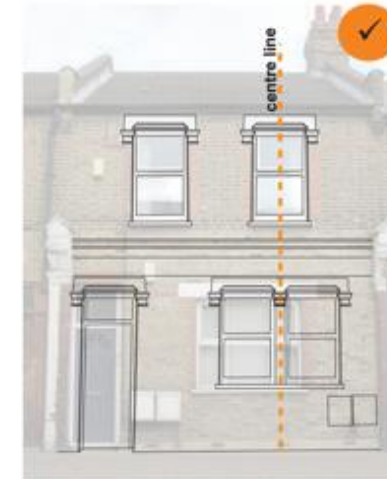
Preferred arrangement. Lower floor windows are aligned with the upper floor and window heads are replicated. The cornice is also retained.
